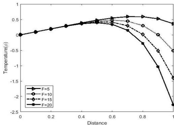
Figure 8: Temperature Profile for various values of Radiation Parameter  $F$ .  $Ga = 0.5, M = 5, K = 0.1$
