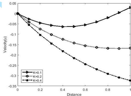
Figure 6: Velocity Profile for different values of Porosity parameter  $K$ .  $F = 5, Ga = 0.5, M = 5$
