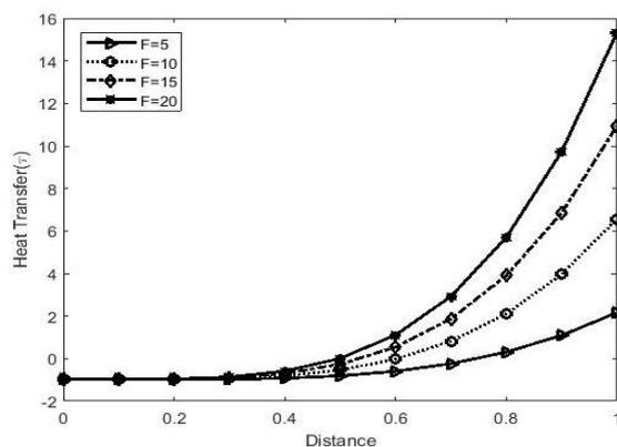
Figure 9: Heat Transfer Profile due to Thermal Conduction for different values of Radiation  $F$
