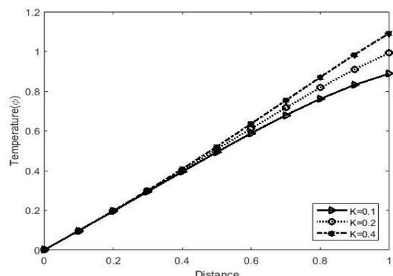
Figure 7: Temperature Profile for different values of Porosity parameter  $K$ .  $F = 5, Ga = 0.5, M = 5$
