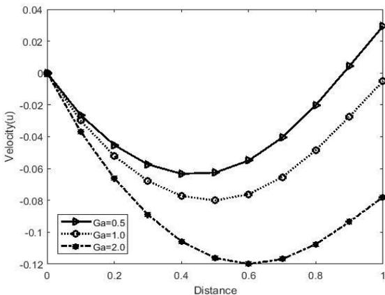
Figure 2: Velocity Profile for different values of Grashof number  $Ga$ .  $M = F = 5, K = 0.1$
