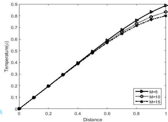
Figure 5: Temperature Profile for different values of Magnetic Parameter  $M$ .  $F = 5, Ga = 0.5, K = 0.1$
