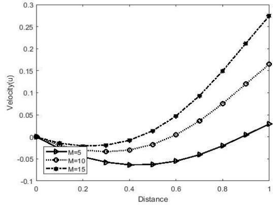
Figure 4: Velocity Profile for different values of Magnetic Parameter  $M$ .  $F = 5, Ga = 0.5, K = 0.1$
