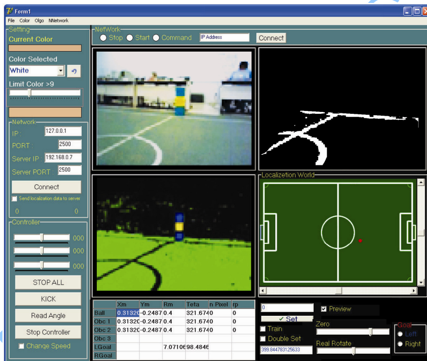
Figure 8. Vision Systems, Object detection (Goals, Flag Spots, Ball) and line detection for Self Localization algorithm
